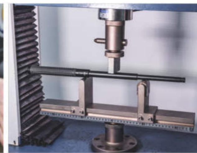
Durability Bending strength \geq 10,000N Tensile strength \geq 1,000N 2m Impact resistant
